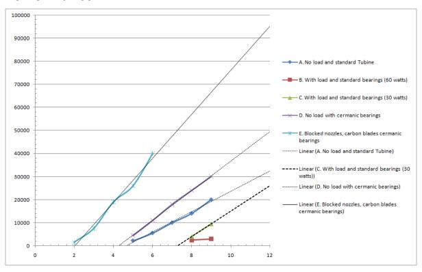
The graph above shows the turbine in a number of configurations. As standard the turbine can spin at the speeds indicated on line A (5 to 9 CFM) and with a bulbs connected 8 to 9 CFM is required to power them, this is shown on line B. Changing the bulbs from 60 watts to 30 watts results in the requirements shown in line C.
